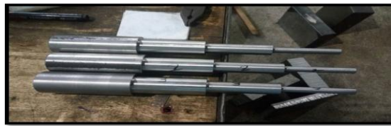
Figure 2: Work pieces processed on CNC Lathe
